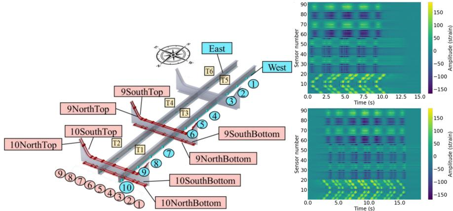
Fig. 1: (left): the location of the three types of sensors installed on the bridge: longitudinal in blue, transversal in red and temperature in yellow [4]. (top right): strain induced by a train passage with 16 axles and in the south direction (N-S). (bottom right): same as (top right) but with 24 axles and in the north direction.
