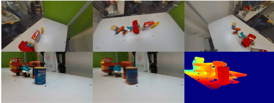
Fig. 3: Top row: Three source views (Input to our model). Bottom left: Target view RealSense image. Bottom mid: Neural rendering for that view. Bottom right: Depth predictions by our model. Note that the geometry of the lower wing is correctly reconstructed despite not being visible from the input views.
