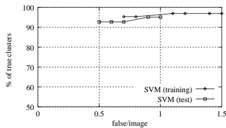
**Figure 4.** FROC of the detection for *training* and *test* with SVM classifier.
