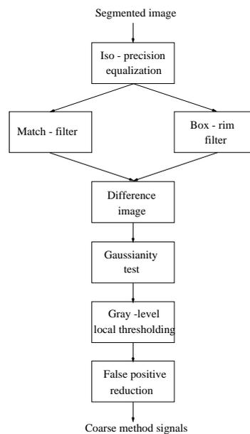
**Figure 1.** Scheme of the coarse method.
