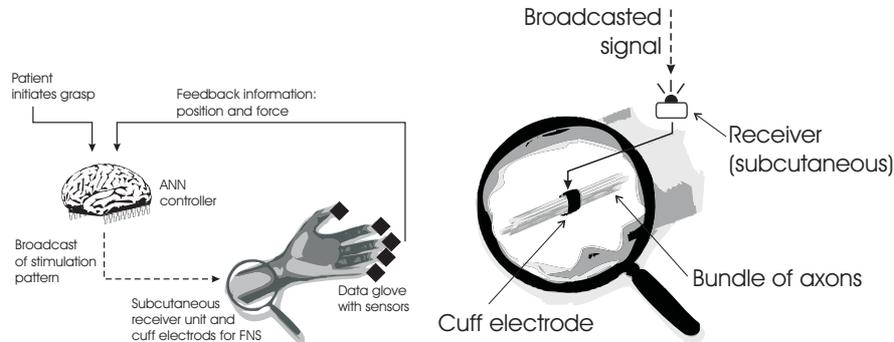
Figure 1: *Left illustration: proposed scheme of the closed-loop system for grasp control. Right illustration: implementation scheme for a subcutaneous receiver unit and the cuff electrode around the nerve.*
