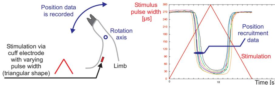
Figure 2: *Left illustration: Setup of the data recruitment experiment. Right illustration: FNS stimulation patterns and seven resulting position trajectories.*
