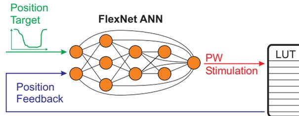
Figure 3: Scheme of the closed loop position control based upon a FlexNet controller. The limb movement is simulated using a look up table (LUT).
