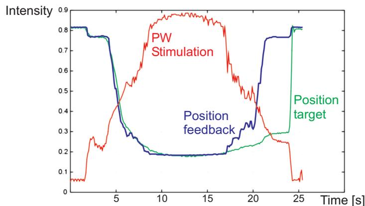
Figure 4: Results of the simulation of closed loop position control. The simulation was carried out as described in figure 3.
