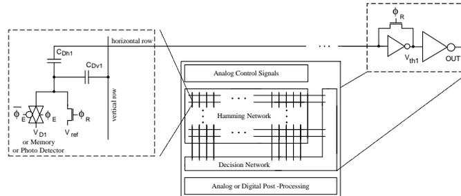
Figure 5: Array arrangement of the Hamming distance classifier.
