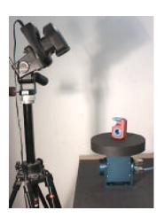
Figure 1: Above: Turn-tilt table for object presentation with active camera. Right: Semi-automatic data acquisition. Automatically selected windows are clustered using a SOM, then the user selects regions of nodes as classes to train a classifier.
