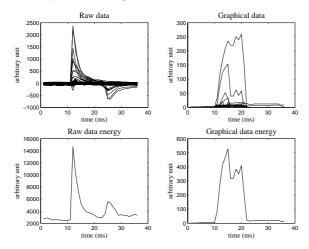
One can see that the onset of the touch is easily detected by thresholding the rising front of the energy signal (with some heuristic rules to prevent jitter). Detection of the release of the fingers is somewhat more difficult, but since we are interested in the classification of the gesture as soon as possible, we cannot wait for the release event anyway.
