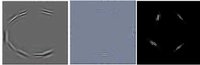
Fig. 4: Example basis functions of Curvelet (the first two) and Countourlet (the last one)
