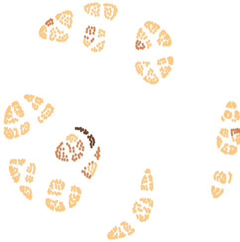
Fig. 4: Reliable and unreliable areas of a visualization using Sammon mapping. Colors correspond to reliability levels. All points are reliably placed in 1–6 clusters; at the next granularity level, about 7–20 clusters, darkest points may be wrong. Medium dark means reliability problems start at scale of 21–50 clusters, and all points more reliable than that are drawn with lightest color.
