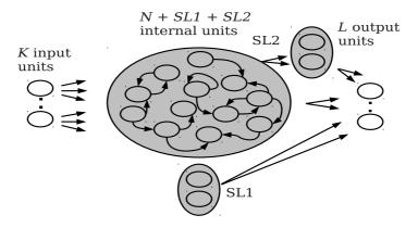
Fig. 1: Reservoir with Random Static Projections (R<sup>2</sup>SP). SL1 and SL2 are the number of neurons in the respective static layers.
