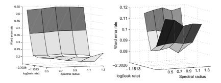
Fig. 2: Test error plots of the standard reservoir (left) and the R<sup>2</sup>SP (right) when applied to the digit recognition task ranging over the leak rate and the spectral radius. Note the different scaling of the Z (error) axis.
