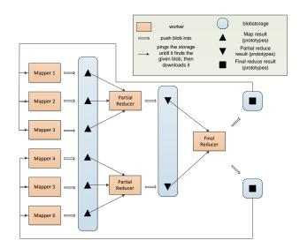
Fig. 1: Workers communication architecture.
