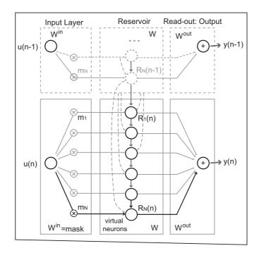
Fig. 1: Schematic overview of the Time-Delayed Reservoir scheme (TDR) with input u, the reservoir  $\mathbf{R}$  and the final output y, resulting from the read-out linear function of the reservoir state.
