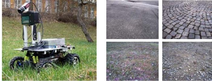
Fig. 2: The mobile robot used for ground image acquisition (left). The four terrain classes used in the ground dataset (right). From left to right and top to bottom: Asphalt, cobblestones, grass, gravel
